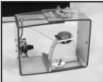
Free-fall demonstration using spring scale.
