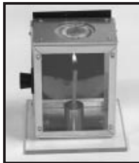
In Earth's gravity, gravity-driven convection rolls cause an easily recognizable flame shape.
