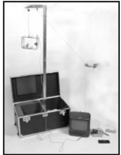
Assembled Microgravity Demonstrator with experiment platform partially raised.
