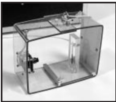
Capillarity demonstration showing effects of microgravity on fluids.
