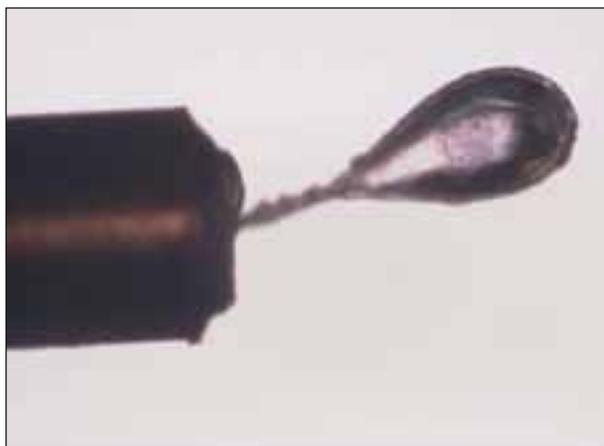
Crystal mounted on a cryogenic loop.
