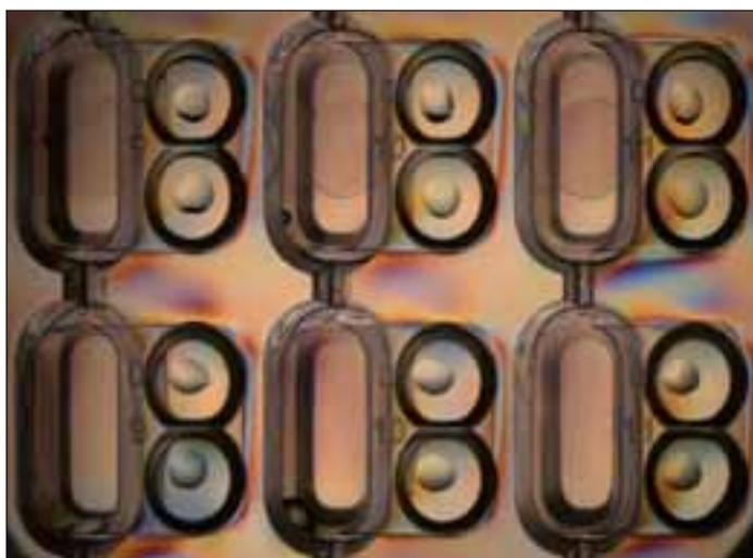
Crystallization drops, pipetted into a microplate by a robotic system, are checked under the microscope for uniformity.
