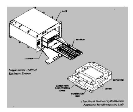
The new PCG hardware consists of a variety of experiment equipment including improved Vapor Diffusion Apparatus (VDA) trays, hand-held Protein Crystallization Apparatus for Microgravity (PCAM) units, the Crystallization Observation System
