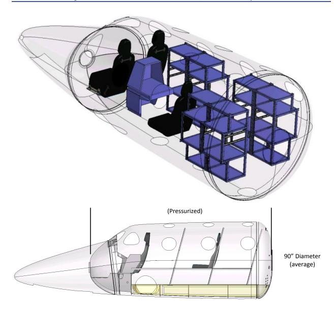
Virgin Galactic has designed a set of payload racks meant to provide support and structure for a wide variety of payloads during flights to space on board SpaceShipTwo. Prototypes of these racks will be installed into and flown onboard WK2 and SS2 in early 2012; any further data or design improvements that result from these tests will be incorporated into further versions of this Payload Users Guide.
