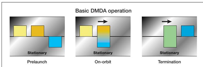
This drawing depicts a cross-section of a set of DMDA specimen wells, one of which can include a reverse osmosis membrane to dehydrate a protein solution and thus cause crystallization. Depending on individual needs, two or three wells may be used, the membrane may be absent, or other proprietary enhancements may be present.
