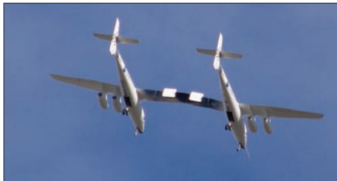
WK2's twin fuselage placement enables the aircraft to carry a multipurpose range of payloads.
