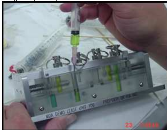
The ITA Materials Dispersion Apparatus (MDA) Demonstration and Training Unit (shown being loaded) is applicable for use on Low-g aircraft or in classrooms or labs as a ground control unit supporting on-orbit experiments.
