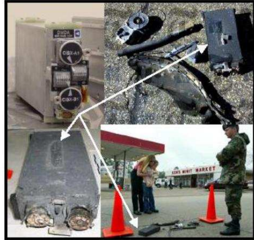
Figure 4. Composite picture of recovered DMDA hardware (containing GOBSS experiment) in Nacagdoches, Texas. February 2003.
